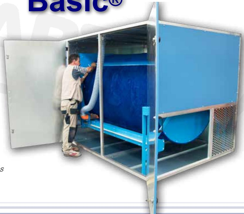
*This family of product is standardized with specific dimensions of the modules to permit to joint the pieces in various shapes and solutions in order to adapt the installation to the available spaces.*
