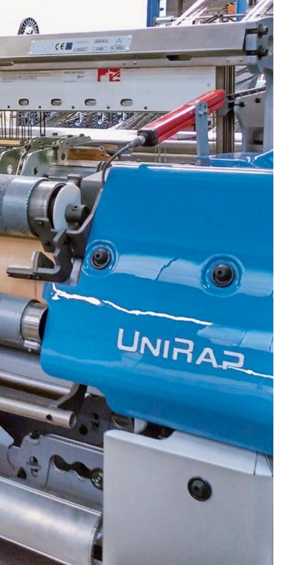
UniRap embodies versatility and provides endless weaving possibilities. Combining the advantages of a positive rapier weft insertion with the gentle yarns treatment ensured by the free fight transfer system, UniRap enables complex and creative fabrics weaving with practically no limitations.
